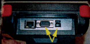
3. A 9 pin "D" connector and a power connector are on the side of the computer.
