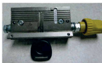
Vise jaw 'G' for cutting automotive double-sided flat keys
